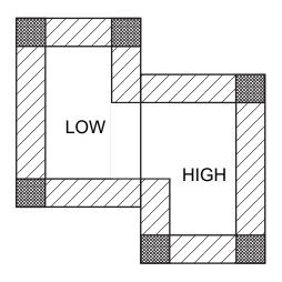
Note: Where multi-level roofs meet at a common wall, the adjacent edge of the upper roof is treated as a perimeter requiring enhanced fastening only if the difference in height is greater than 3 feet (90cm). Neither Lexcan nor FM requires fastening enhancement at the lower roof area adjacent to the higher building wall, regardeless of height differential.
